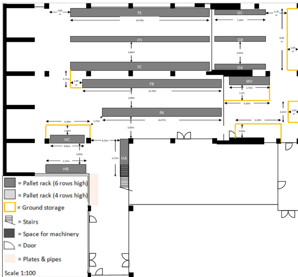
Figure 11: Measurements of aisles and storage places of the current layout in Publisher
