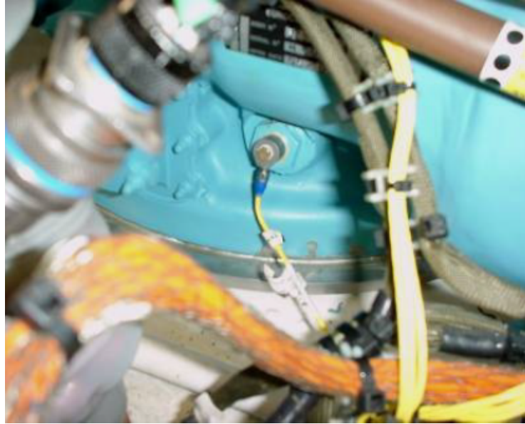
FIGURE 2.3 – Accelerometer on the shell of the MGB of the EC225 (EUROCOPTER, 2012)
