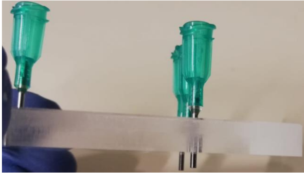
Figure 16: Top part of mini-FCB where blunt needles went through the PMMA.
