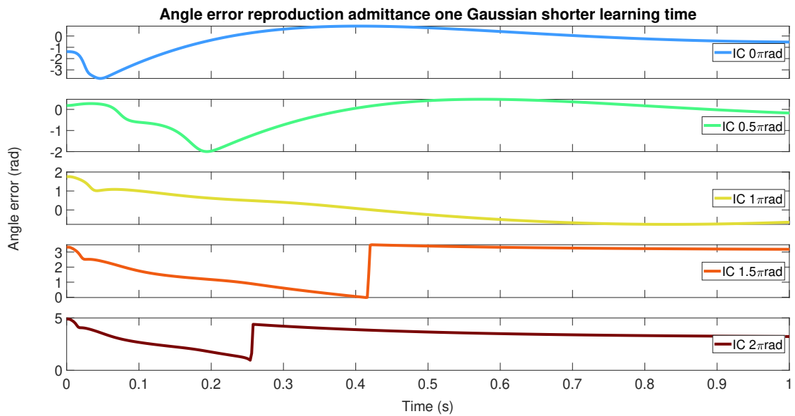
Figure C.3: The angle error [rad] between the reproduction of the one Gaussian GMM with shorter learning time and admittance controller for the interpolation initial conditions of the mass angle.
