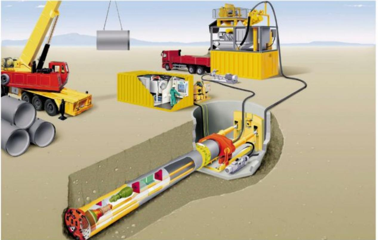
**Figure A.1:** Example of microtunneling and its excavation [33]
