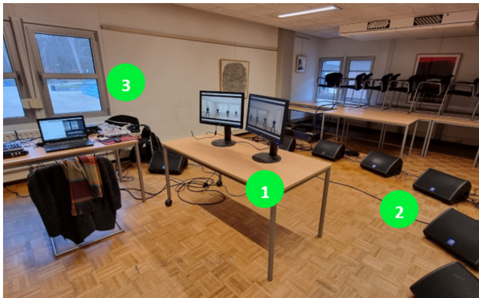
Figure 5.4: Experiment setup: 1) two-screen video setup, 2) half-circle audio setup, 3) haptic wearable station
