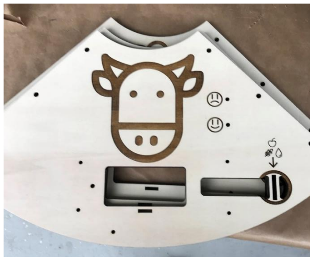
Figure 29. The lasercut animal zone parts. The holes on the sides allowed the parts to be easily attached to the table base using screws. Similarly, the holes at the bottom allowed the object deposits to be attached to the animal zone parts.
