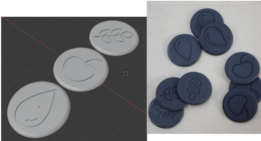
Figure 14. On the left: 3d model of the final food object coin designs with inset food type icons. On the right: the final 3d printed coins of the prototype
