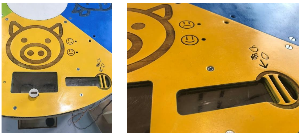
Figure 18. The food deposits on the prototype table. On the right above the object insertion slot there are the food objects with an arrow pointing to the slot. All the icons on the table are engraved into the table top.
