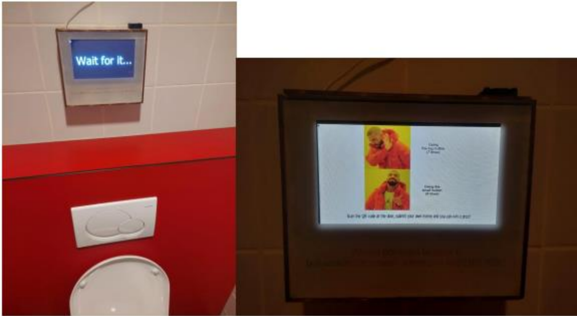
Figure 13: The meme screen, a solution for making toilet users more aware of their flushing behaviour. (Kadijk, 2021).
