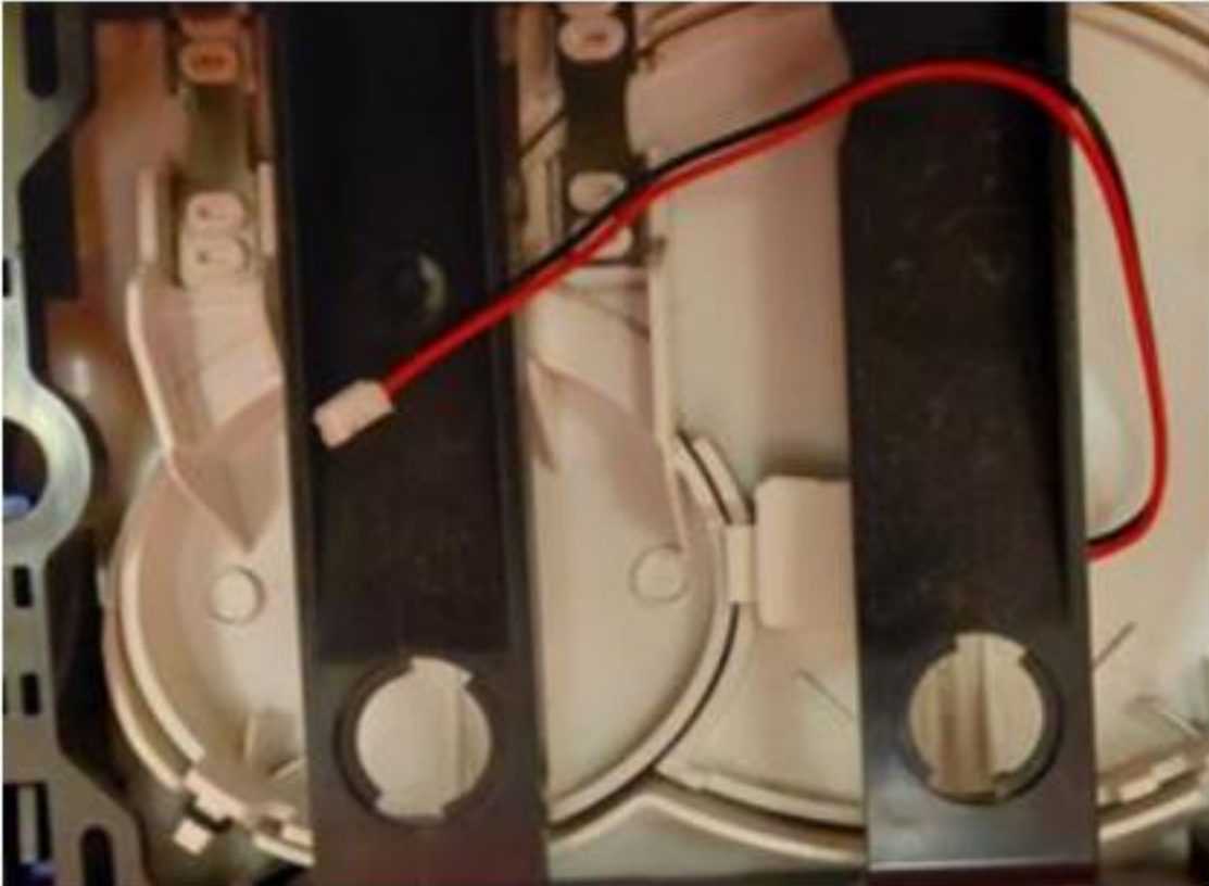
Figure 7: Implementation of a Piezo sensor behind a toilet button in order to sense when that button is being pressed. (Kadijk, 2021)
