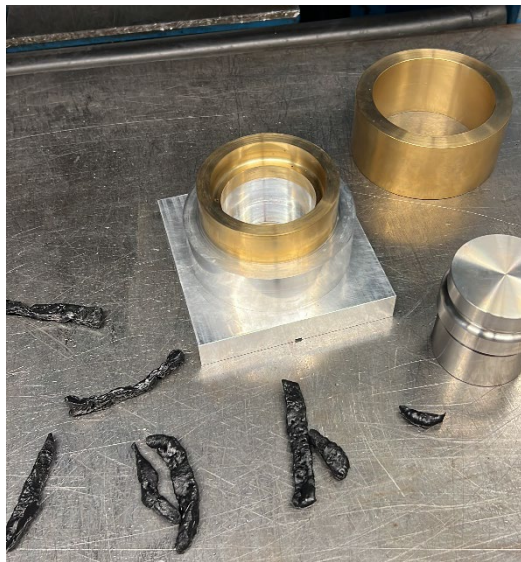
Figure 46: Mold and rubber before curing
