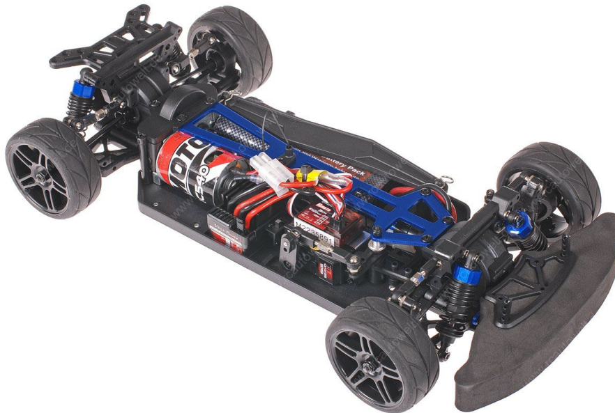
Figure 12: The Himoto Nascada 1/10 used as basis of this project (20)
