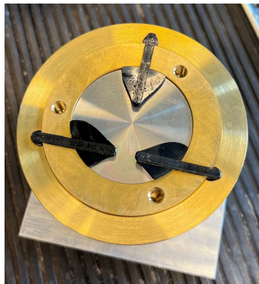
Figure 45: Rubber from relief channel
