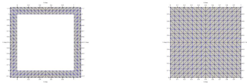
Figure 9: Meshes for the solid domain (left) and the fluid domain (right) for N = 2 .
