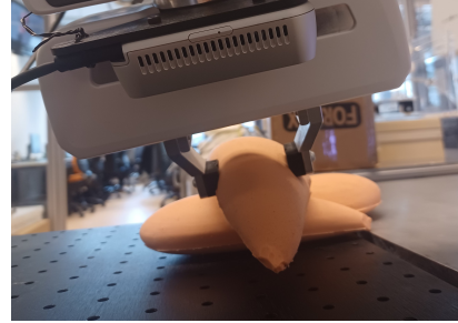
Fig. 15: Executed grasp for chicken fillet in Fig. 11m. The grasp is too high, resulting in the fillet to slip from between the finger grippers.
