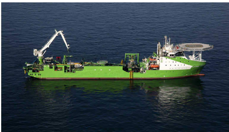
Figure 13.1: Living Stone is a DP3 cable installation & multipurpose vessel Source: (DEME Offshore, 2022)
