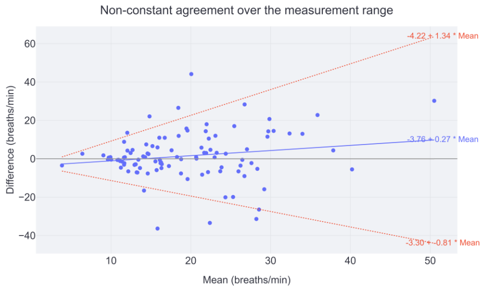
Figure 2. Example of a Bland-Altman plot with a non-constant agreement in respiratory rate measurements. The variability increases with the mean of the respiratory rate. The regression of difference LoA analysis represents the systematic relationship between the difference and mean.
