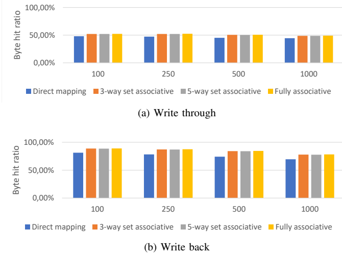
Fig. 9: Byte hit ratio for different cache organizations using a cache with 32 lines and LRU replacement policy.
