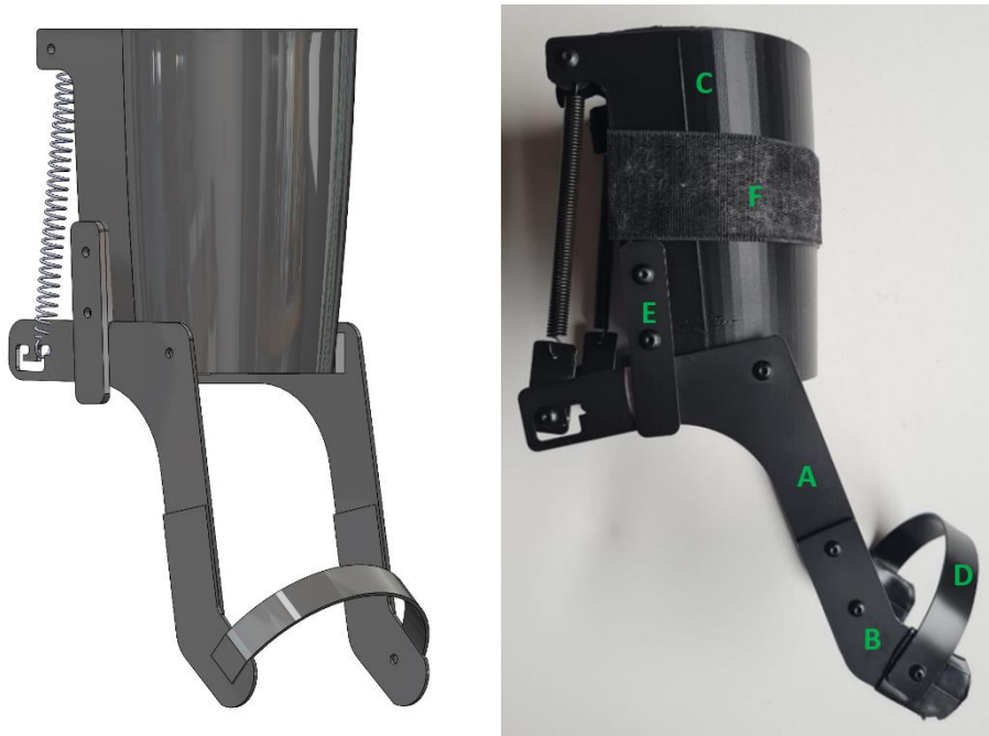
Figure 12 Left: front view of the Solidworks drawing of the prototype. Right: construction of the prototype without the back shell, with A) The lever, B) the bent end of the lever with the anti-slip material, C) the attachment to the lower leg, D) The extra band at the end of the levers, E) the mechanical stop and F) the Velcro to connect the two shells together.
