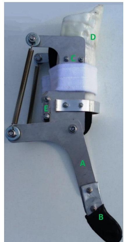
Figure 3 The previous design with A) The lever, B) the bent end of the lever with in black the anti-slip material, C and D) the attachment to the lower leg with padding in D and E) the mechanical stop
