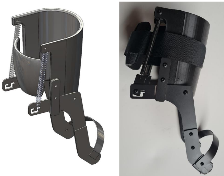
Figure 13 Left: back view of the Solidworks drawing of the prototype. Right: construction of the prototype with the back shell attached.
