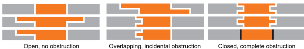
Figure 7: Overview of Assembly Shape types copied from (Dutch Green Building Council, 2021a)
