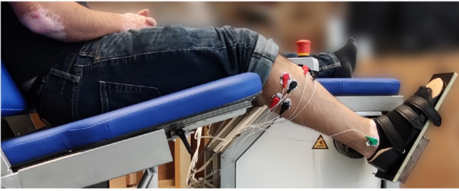
Fig. 1: Electrode and marker placement on the subject during the experiment in Achilles to determine ankle stiffness. Figure adapted from [9]
