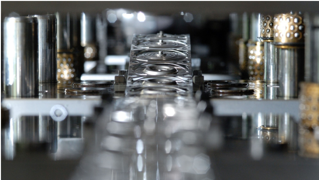
Figure 1.1: The deep drawing process of the shaving caps in Philips Drachten.
