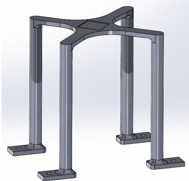
**Figure B.3:** SolidWorks design for the platform on which the designed workspace is placed. This platform is placed inside the BatMag system.
