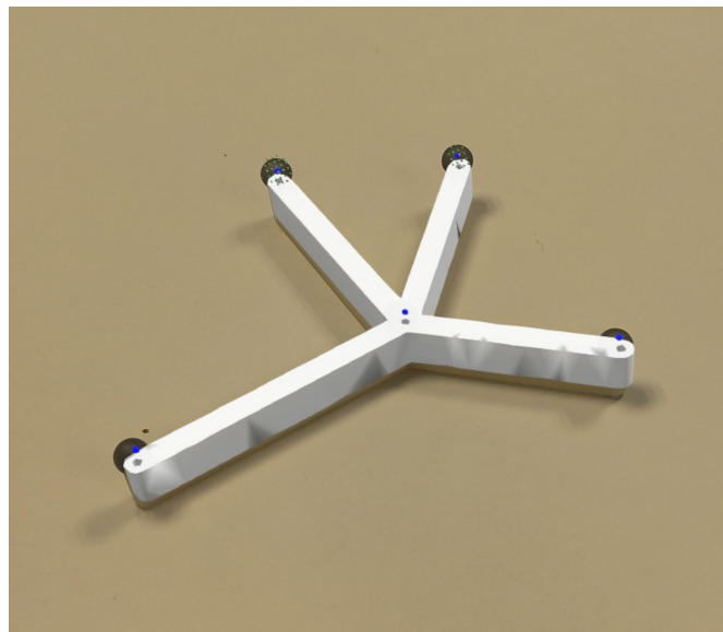
Figure 22: Holographic display of the reference star. The center point of the IR markers is shown as blue dots
