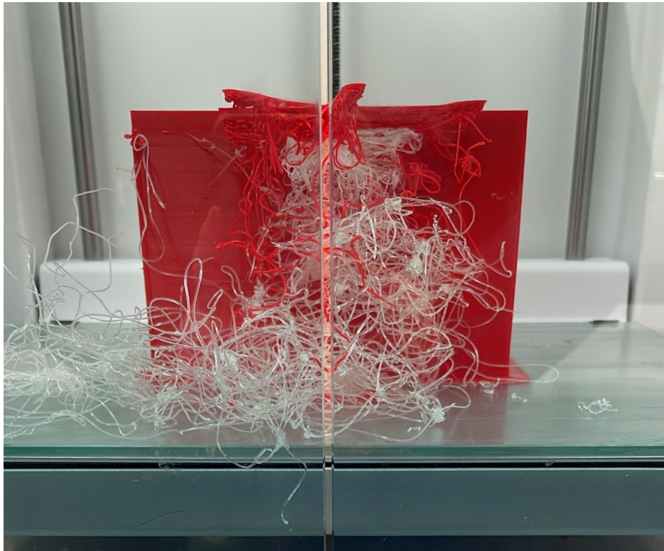
Figure 37: Failed 3D print with PLA and PVA in the 3D printer
