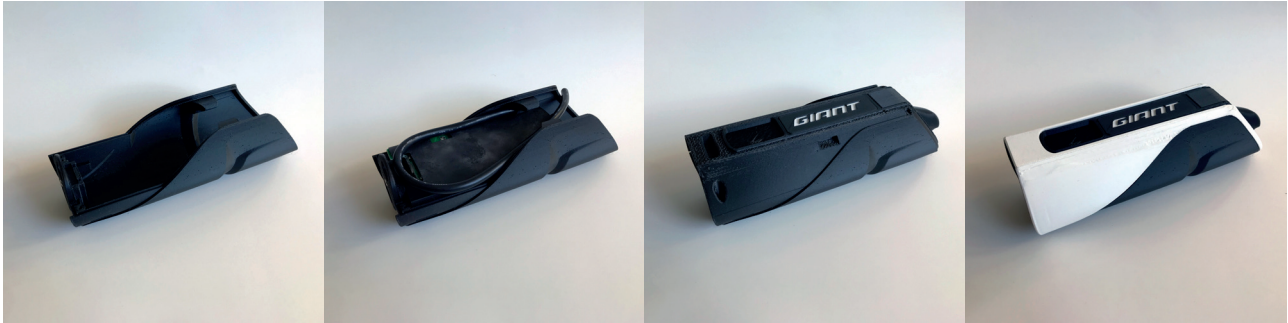
Figure 229: Assembly process of the portable charger
