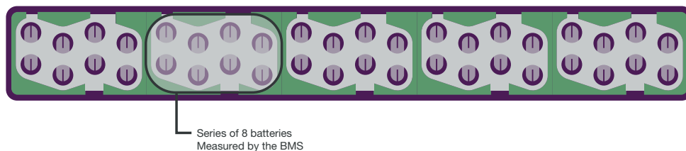
Figure 126: Internal structure of one of Giant's Batteries [1]
