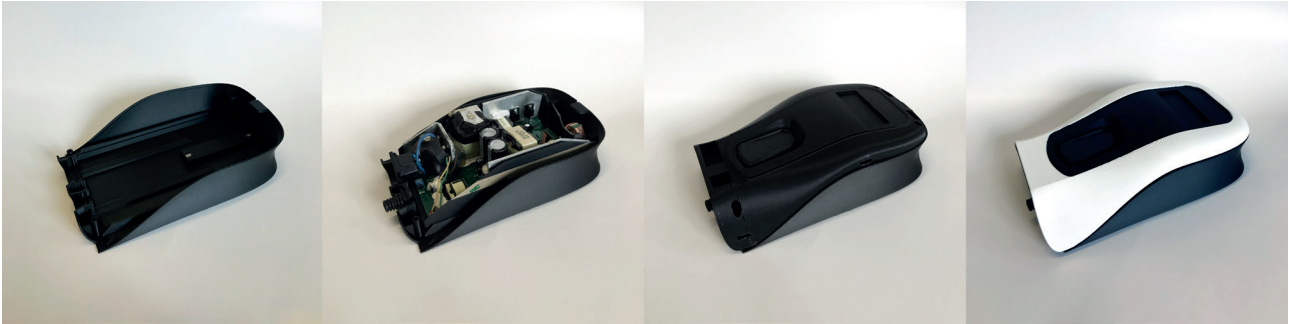
Figure 221: Assembly process of the home charger
