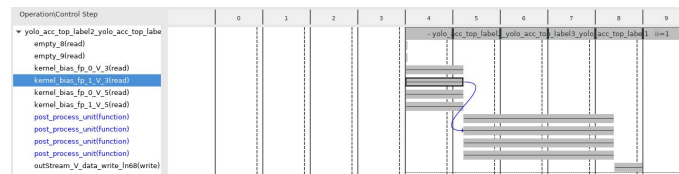
Figure 4.7: Loop 2 improved initiation interval with pipelining and memory partition: solution 3
