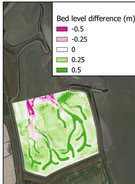
Figure 5.1: Bed level difference between 2016 & 2022 in the intertidal area of Perkpolder managed realignment site. North of bed level differences lies the deep pond.
