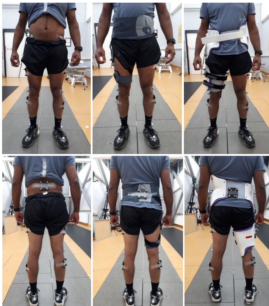
Fig. 2. Marker setup for the biomechanical gait analysis during the three examined conditions. From left to right: 1) Marker set without wearing a hip brace, 2) with the Rebound hip brace, and 3) the Newport 4 hip brace.
