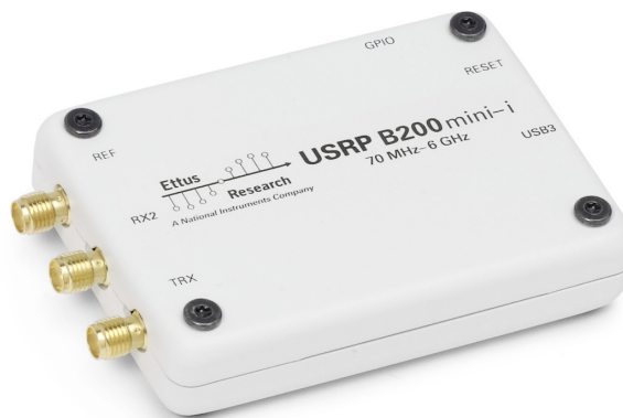
Figure 2.5: Photo of the universal software radio peripheral (USRP) B200-mini software-defined radio. From [23].
