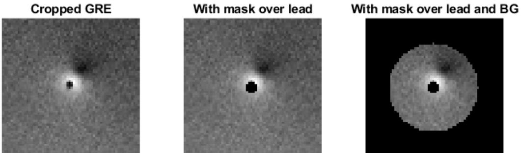
**Figure 3.6:** The three different ways of fitting: cropped GRE pre-scan image, with the addition of a mask over the lead, and a mask over the lead and background.
