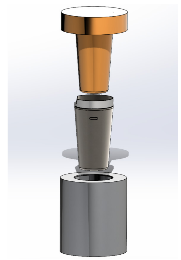
Figure 189: Exploded view injection mould to edge
