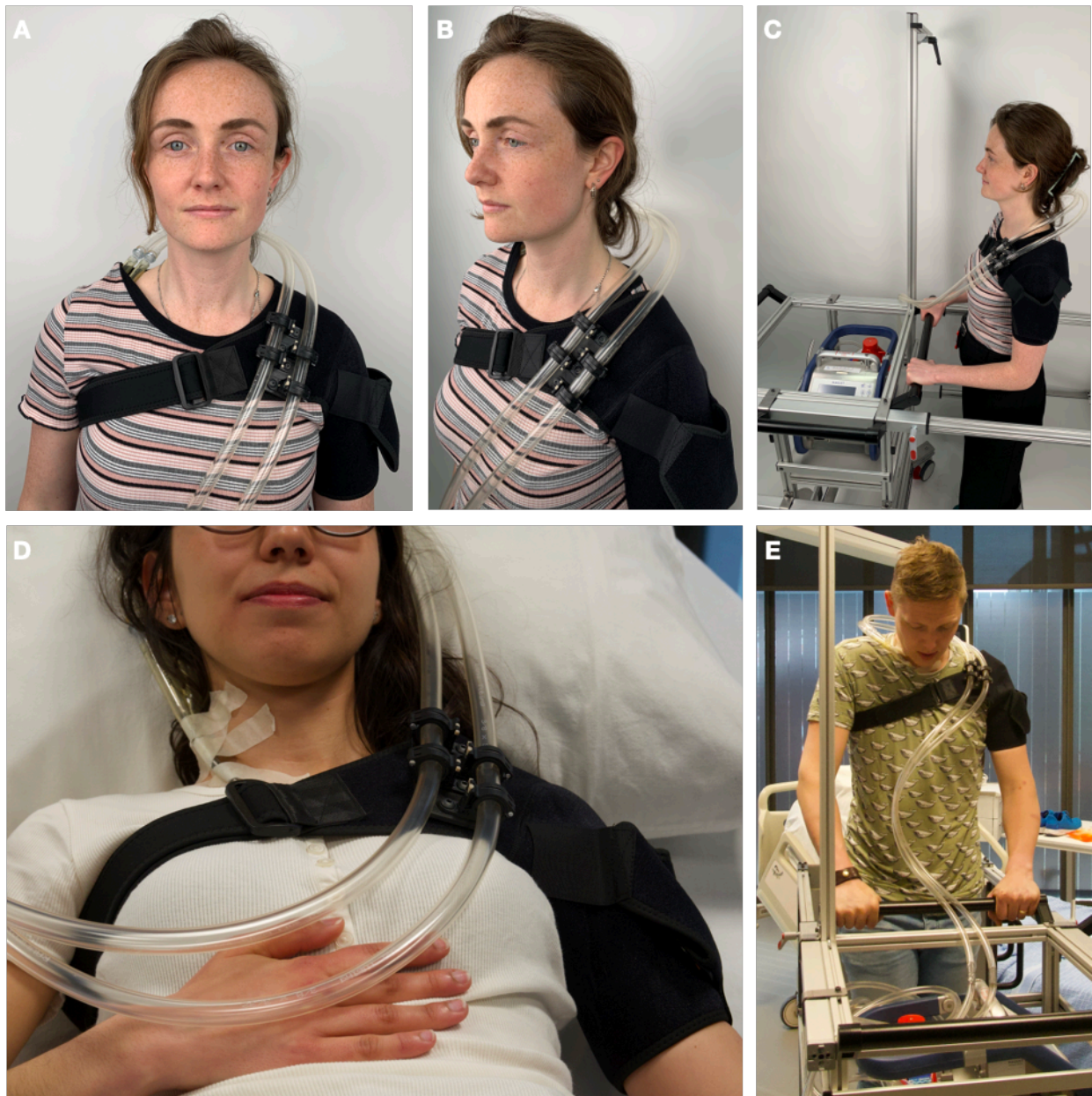
Figure 7: Simulated ECMO patients wearing the blood tubing fixation module prototype during (A-C) a static standing position, (D) lying in bed, (E) walking with the ambulatory cart
