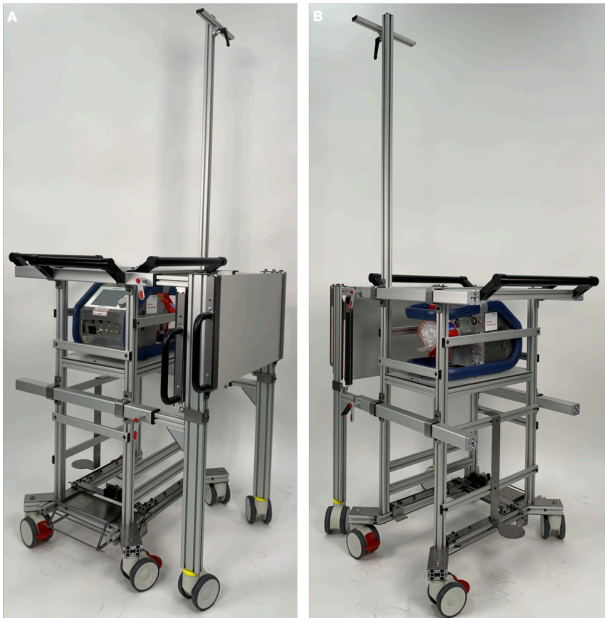
Figure 9: (A) front view and (B) rear view of the prototype of the ambulatory device transport module which provides transport of devices necessary in both stationary and ambulatory conditions
