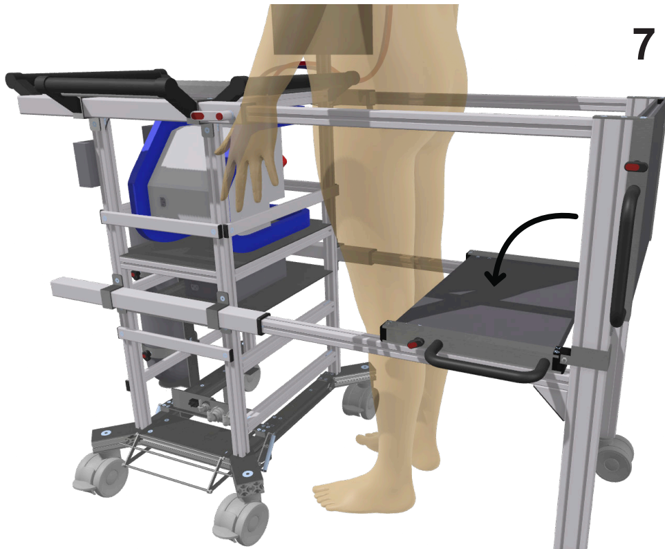
Figure 23: User scenario, step 7 – In case of patient fatigue, the foldable seat enables the patient to sit down. The caregiver unfolds the seat and assists the patient.
