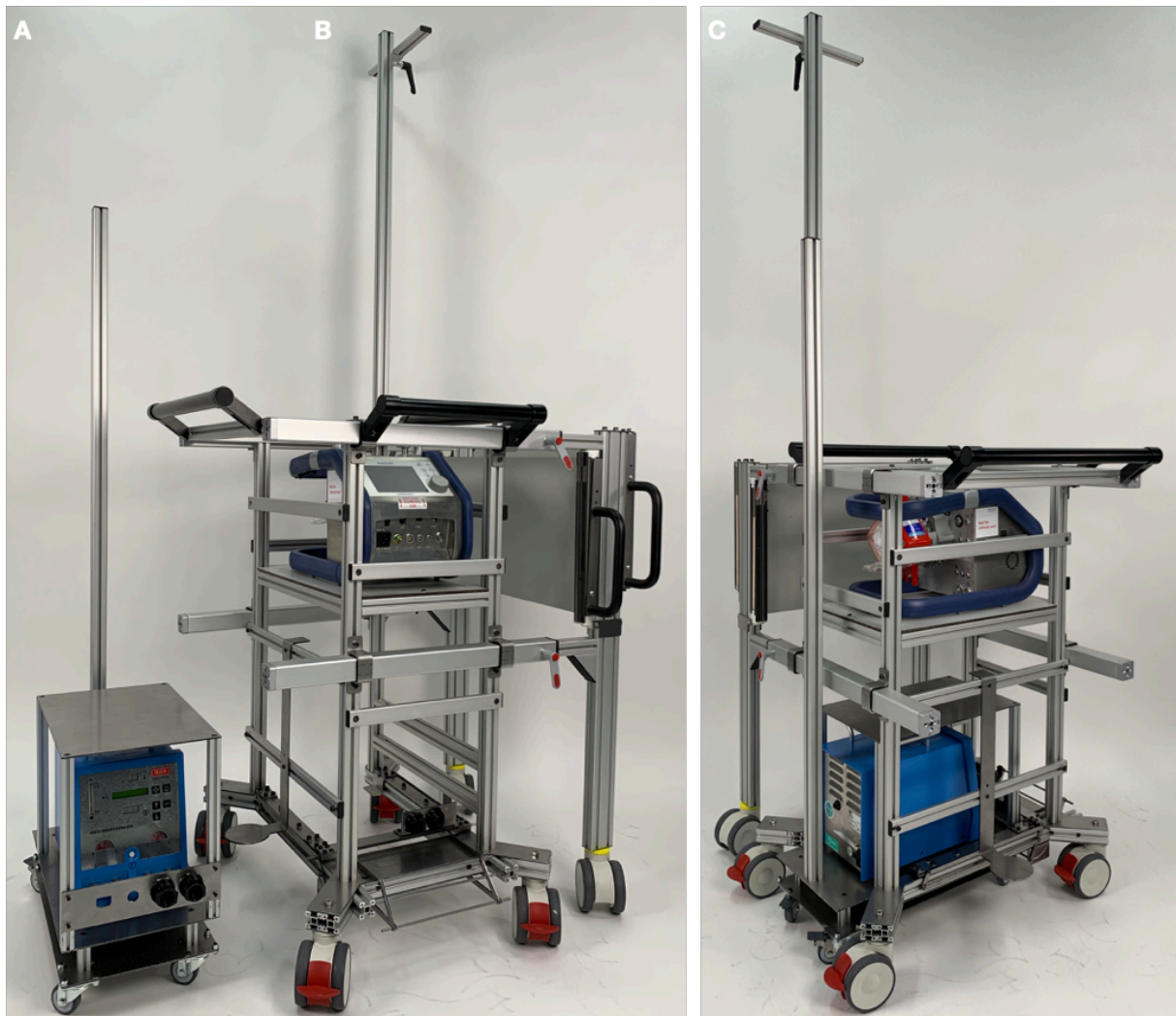
Figure 11: (A) Prototype of the stationary device transport module (left) providing transport of devices only necessary in stationary conditions, (B) prototype of the ambulatory device transport module, (C) Ambulatory ECMO cart combined with the stationary cart as used in stationary ECMO conditions
