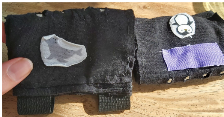
Figure 6.4: Final iteration of the I-Five showing the two markers on the reader (seal) and tag (penguin), and the colour of the LED that this wristband can give (purple).
