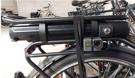
(a) The action camera is mounted to the side of the carrier on one bicycle
