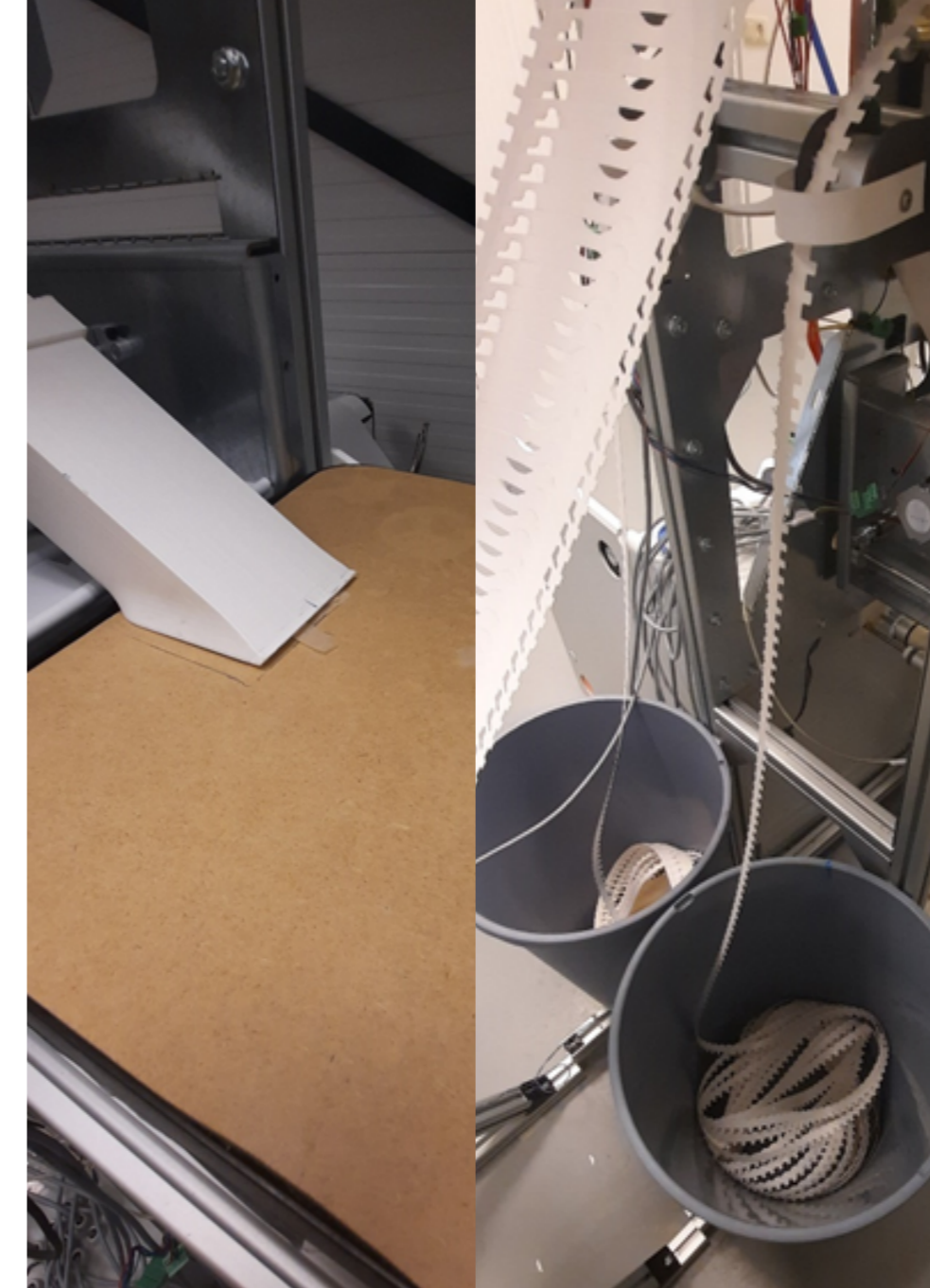
Figure 48: Outflow of waste material: filter paper (left), cartridge waste (right)
