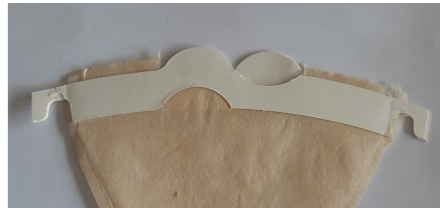
Figure 61: Too large of a shift in module 60 resulting in problems with placement of bracket
