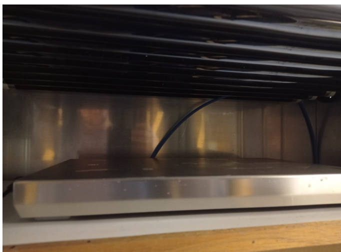
Figure 10: Picture of the setup used for illumination of samples using UV light. A row of 8 lamps of 18 W can illuminate samples from above on a plate with 4 x 5 magnetic stirring spots.
