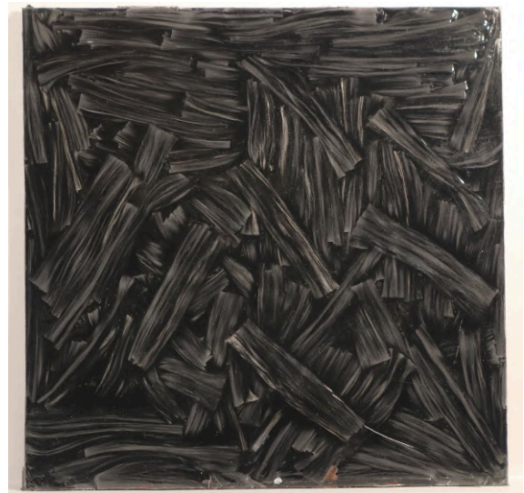
(b) Random pellet configuration after pressing
