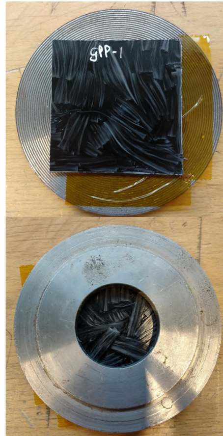
(b) Specimen (60x60 mm) on clamping surfaces. The \varnothing 40 mm impact zone on the lower image.
