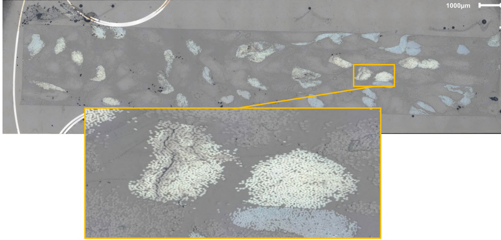
Figure 5.3: Matrix cracking inside a Twaron fiber bundle
