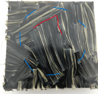
(e) Specimen G/A/PP-1.4 fracture on bottom side
