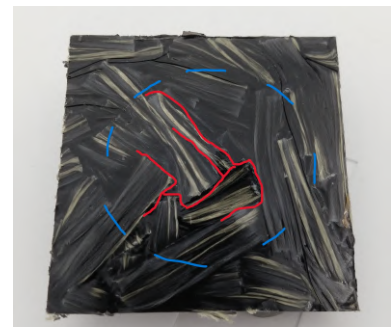
(f) Specimen G/A/PP-2.1 fracture on bottom
