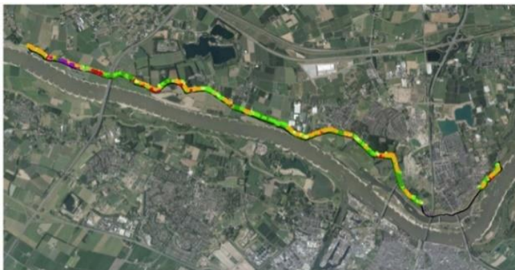
Figure 3. An image containing the overview of the studied Waaldijk. The image shows the result of the piping assessment. Green is safe, others are unsafe. (van de Stroet & Rouash, 2020)
