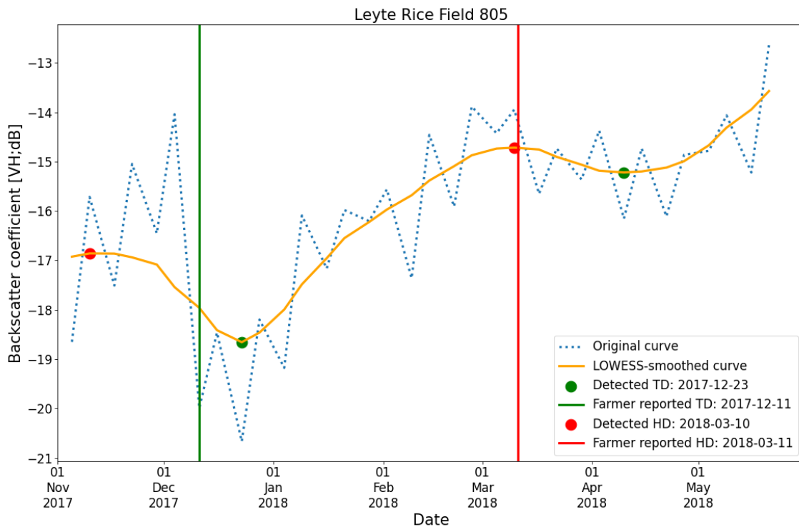
Figure 4.9 SAR VH backscatter coefficients and LOWESS-smoothed time series curve with farmer-reported and detected dates for field 805 in Leyte during the dry season
