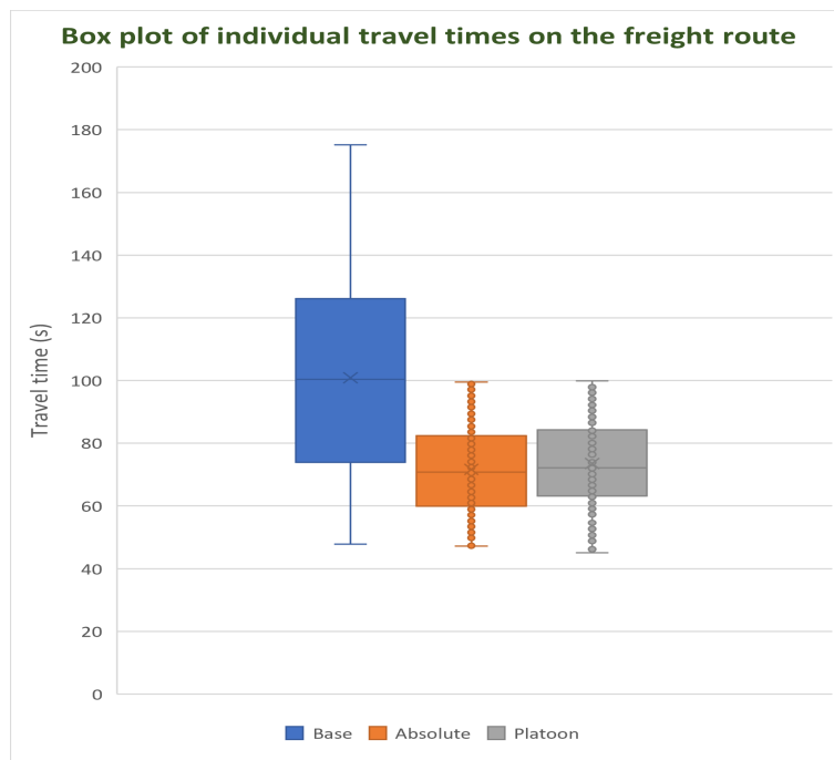
FIGURE 4.9: Box plot for individual travel time of trucks on the freight route for each priority strategy (peak period)
