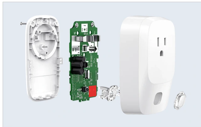
Figure 19: Hardware overview of Moko MK107 gateway, the WiFi-BLE antenna is located on the backside of the PCB, at the red marked position. Adapted from [1].
