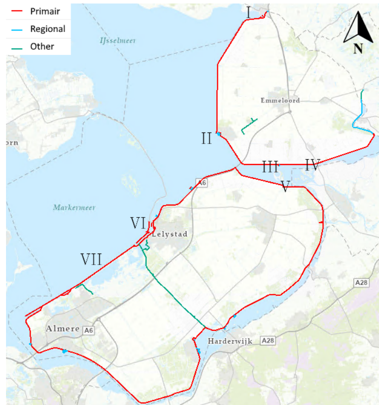
Figure 1.3: Location of breakwaters in Zuiderzeeland control area. Primary flood defence structures provide protection against external water from the Northsea, Waddensea, the main rivers and the IJssel- and Markermeer. Regional flood defence structures provide protection against internal water from the rivers and canals [3]. Structures labeled as 'other' do not provide direct protection against water, but have been doing so in the past or might be in case the primary structures fail. A brief description of each case can be found in Table 1.1. Roman numbers in the figure correspond to the numbering in the table.
