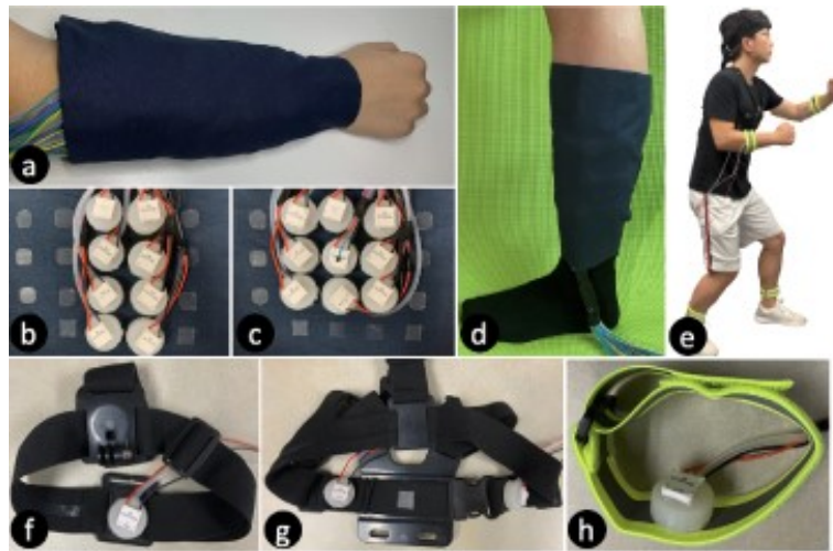
Figure 7: Multiple use cases of the PnueMod [53]. a) Sleeve worn on the forearm and d) on the lower leg. h) An actuator attached to a band that can be worn like in e).
