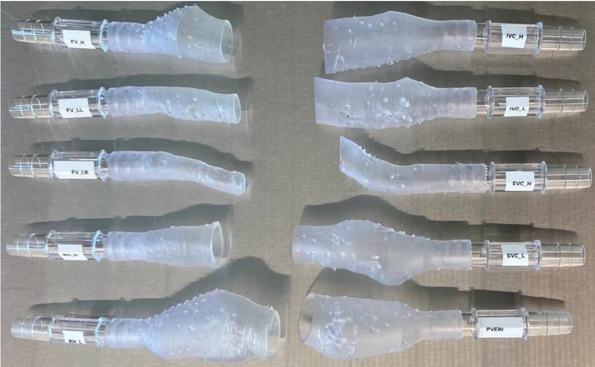
Figure 12-12: Test vessels. Printed with Form 2 SLA printer and Elastic 50A V1 resin. They can be used for testing connectors.
