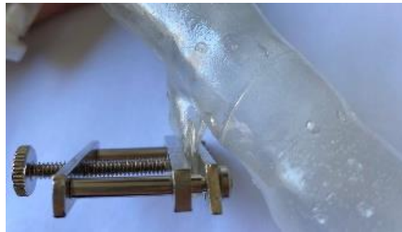
Figure 4-12: Pinchcock clamp causing tears in branch of cannulation path.
