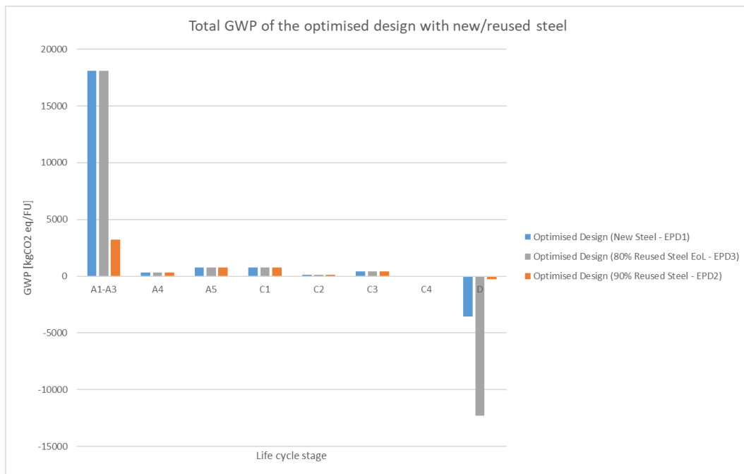
Figure 18: GWP of the entire optimised design made with new and reused steel elements based on EPD1,2,3.
