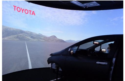
Fig. 4: Driving simulator at Toyota Motor Europe, Belgium
