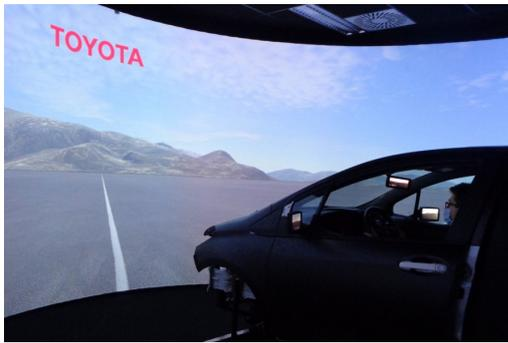
Figure 4. Driving simulator at Toyota Motor Europe, Belgium
