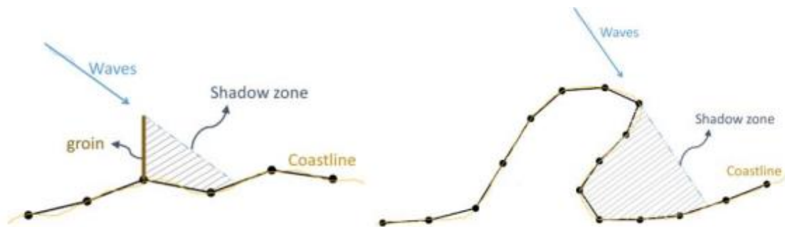
Figure 4: Areas affected by wave shadowing the case of a hard structure or coast section
