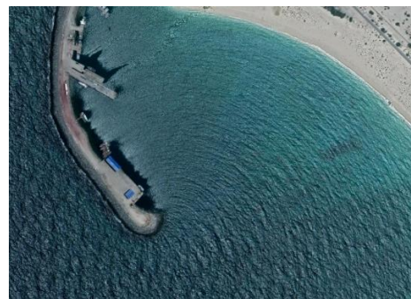
B: Wave diffraction around the tip of a breakwater.
