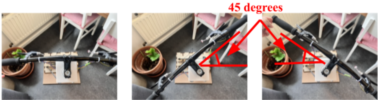
Figure 7.4: limited range of steering angle (45 degrees).
