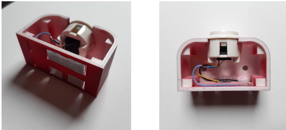
Figure 21: Button element opened
