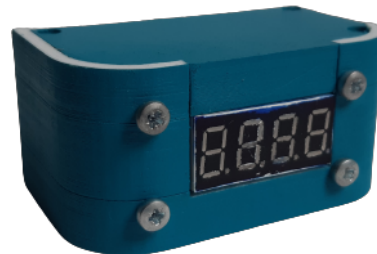
(b) Final 7-segment display element
