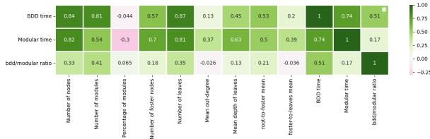
Fig. 13. Pearson correlation coefficient between the logarithm of the computation times of the algorithms and the graph attributes
