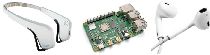
Figure 29: Hardware used for lo-fi prototype version 2 (muse [41], raspberry PI, earphones, and laptop)
