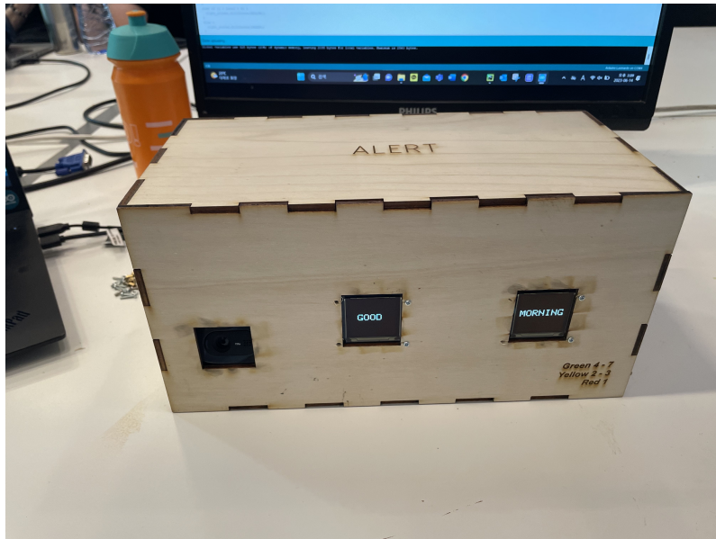
Figure 45. The wooden box including the webcam and two screens
