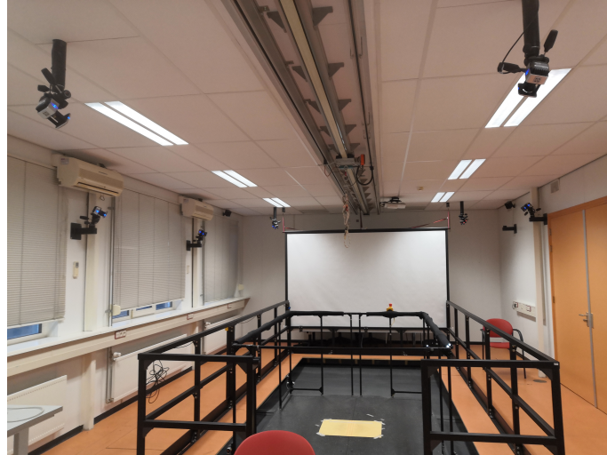
Figure 5: A photo of taken of the motion capture setup used during the recording session. Shown are some of the Vicon Vero cameras, the white screen facing the balance platform and the white mat representing the middle of the platform.
