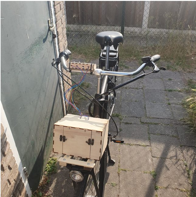
Fig. 9. Data collection setup attached to the e-bike.
